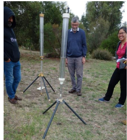
Student briefing and a Guelph Permeameter at work, drip, drip, drip (it's how fast it drips that tells the story)
